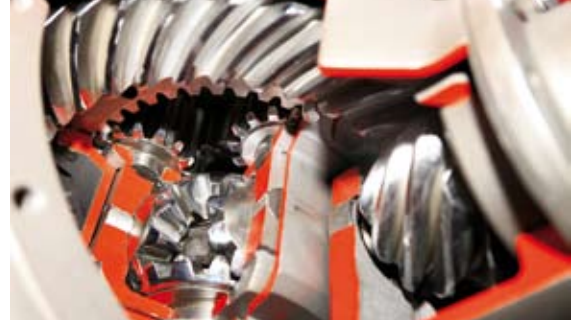
The planetary gearset built into the crown wheel lends it additional rigidity — and resistance to abuse.
